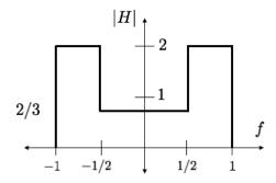
Find the output of this system when the input is  $g(x) = \operatorname{sinc}(x) + \operatorname{sinc}(2x)$ .
