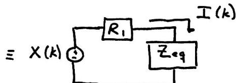
$$Z_{eq}(k) = \left( \frac{1}{Z_L} + \frac{1}{R_2 + Z_c} \right)^{-1} = \frac{Z_L(R_2 + Z_c)}{R_2 + Z_c + Z_L}.$$
