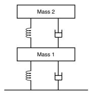
The vehicle is traveling to the right at a known speed. If we consider the altitude of the ground as a function of time x(t) as the input and the altitude of the load as a function of time  $y_2(t)$  as the output, then this is a system. Is this system linear? Is this system causal? Is this system shift invariant? Justify each of your answers.
