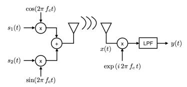
The low-pass filter has a cutoff frequency equal to the band-limit of the two functions. (Assume an ideal low-pass filter throughout this problem.)
