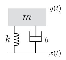
The force due to the spring is:  $F_s = k(x-y)$  .
