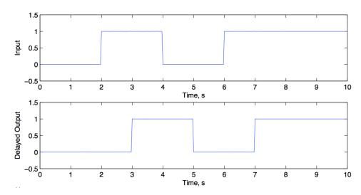
Since the signal arrived out of our system with just a delay, we describe the signal as *distortion free*.
