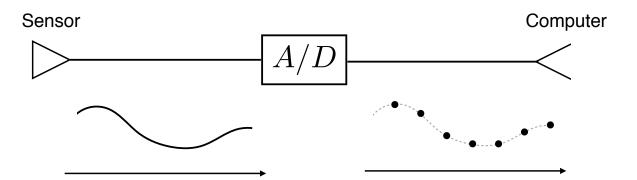
The A/D converts a continuous function into a series of numbers that are then stored in computer memory.
